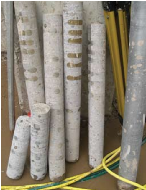
Some of the cores extracted from the basement.
