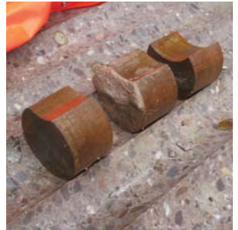
100mm steel plate drilled with an AERO® Core Drill.
